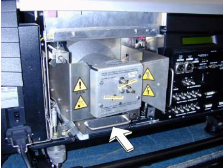
Image 3-11 Inserting the lamp
