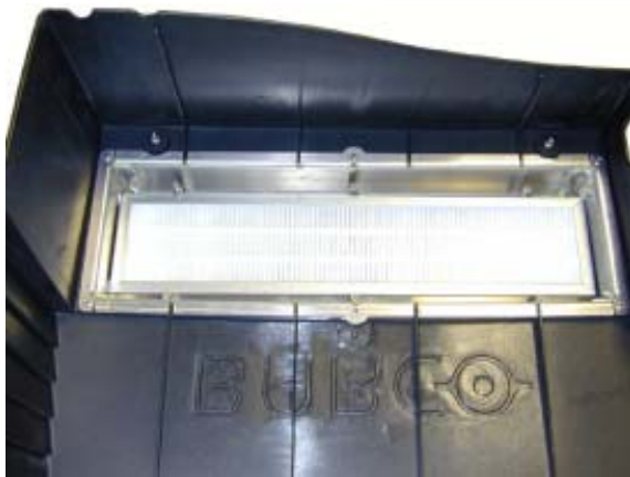
Image B-6 Pull out dust filter and insert new one
