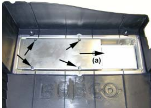
Image B-5 Removing dust filter
