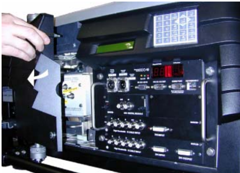
Image 3-9 Pull and remove the side cover
